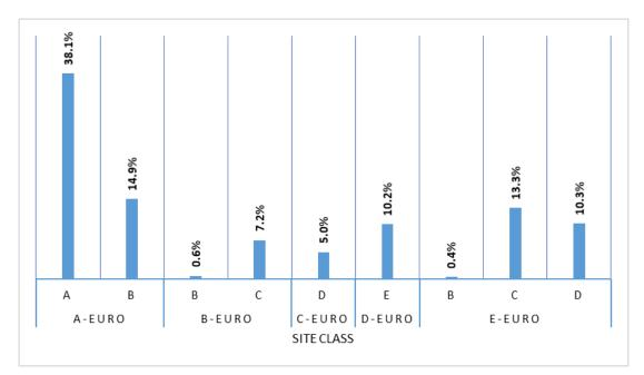
Figure 3. Comparison between Eurocode 8 and NBCC 2015, (NEHRP 2015), site classification for the Saguenay region (the percentage values are based on the area portion of each site class)
