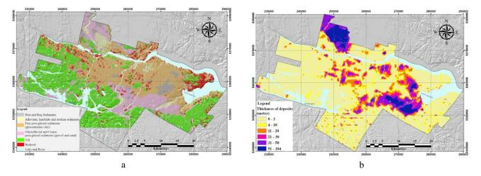
Figure 1. (a) The simplified surface geological map of Saguenay region (modified from [21]), (b) The thickness map of surface-deposits
