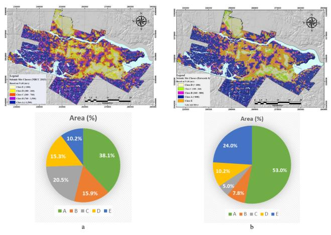
Figure 2. Relative surface area for seismic site classes in the Saguenay region: (a) NEHRP and NBCC 2015, (b) Eurocode 8
